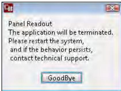
**Communication Error between the Firmware and the Server:** If there is any loss of communication between the embedded controller firmware, the following error message will display on screen. Loss of communication can be caused by a damaged, unplugged or loose embedded controller cable, or when the Emergency Stop button has been pressed. The “CB Scanning Device” Acquisition software will terminate. Check cables and E-stop and restart the system.
