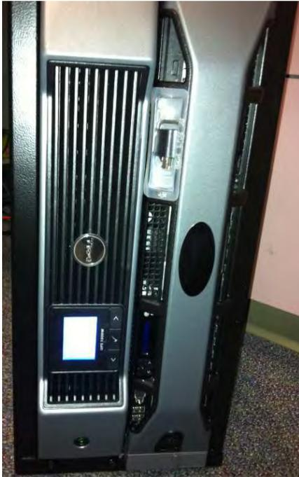
Remove the left cover from the bottom clip. Connect the battery plug. Turn the UPS ON with the button below the plug and verify that it is powered. Replace the cover.
